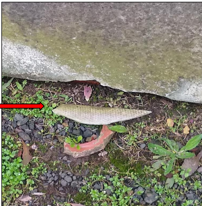
Photograph 3 - Suspected fragment of ACM observed in the south eastern portion of Site A.
